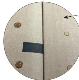
The board on the left absorbs water quickly, which indicates the adhesive most likely will have ideal bond strength. The board on the right doesn't absorb water as quickly and therefore the adhesive will have weaker fiber tear.
