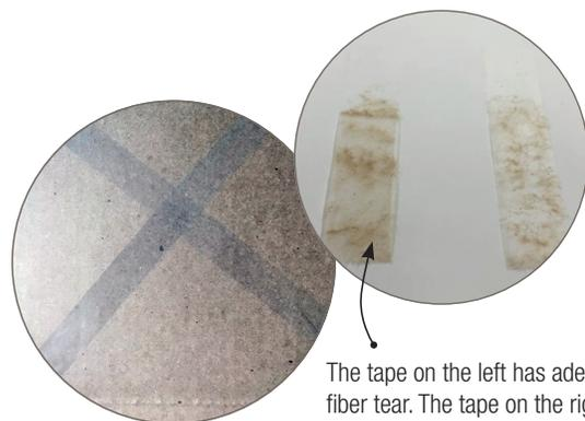
The tape on the left has adequate fiber tear. The tape on the right indicates a difficult board, which will require a robust adhesive with superior bond strength.
